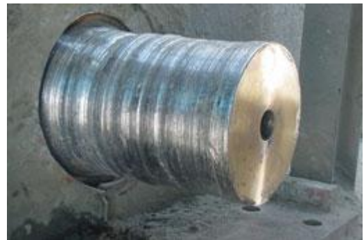
Damage to the Shaft
