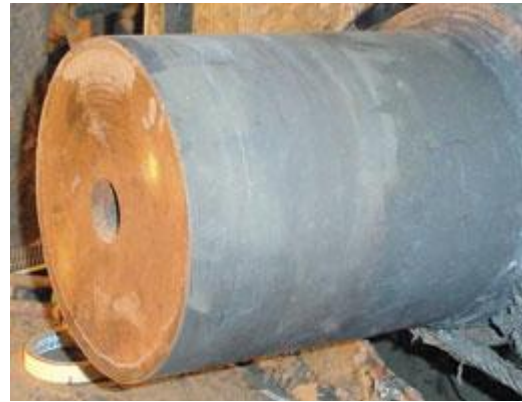
Accurate diameter restored to the shaft
